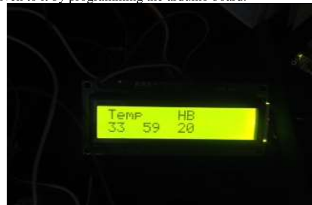
Fig 2 : Heart beat Reading displayed on LCD
