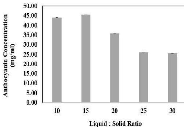
**Fig. 3 Effect of amount of solvent and flower powder ratio on anthocyanins extraction efficiency.**
