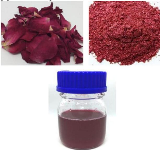
**Fig. 5 Dried Rosa-damascena, pedal powder after milling and red pigment color solution.**
