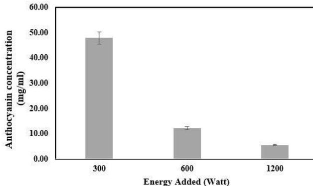
**Fig. 4 Effect of energy power from microwave extractor on anthocyanins extraction efficiency.**
