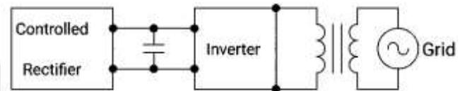
**Fig. 3: Block Diagram of Back to Back Converter [23]**
