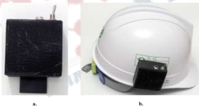
Figure 5: The Designed Sensor tag Housing with Safety Helmet
