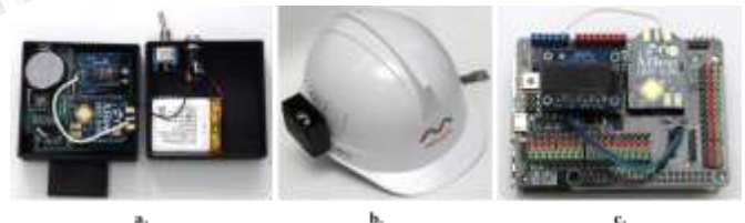
Figure 1: The Developed Sub-1GHz ZigBee based IoT Sensor tags and Routers (a. Sub-1GHz ZigBee based IoT Sensor tag, b. A safety helmet which attached with the sensor tag, c. Sub-1GHz ZigBee based IoT router)
