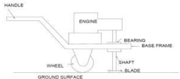
**Figure 1. Grass mower setup.**
