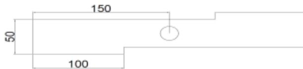
**Figure 2. Cutter blade and its dimension.**
