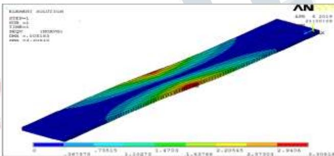
**Figure 3. Von mises stress developed on cutting blade.**
