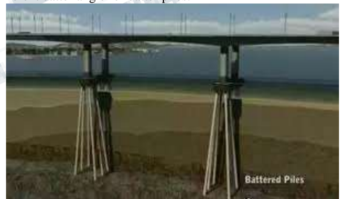
Fig. 1 Batter piles under bridge pier
