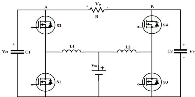
**Fig.1. DC-DC-AC converter**
