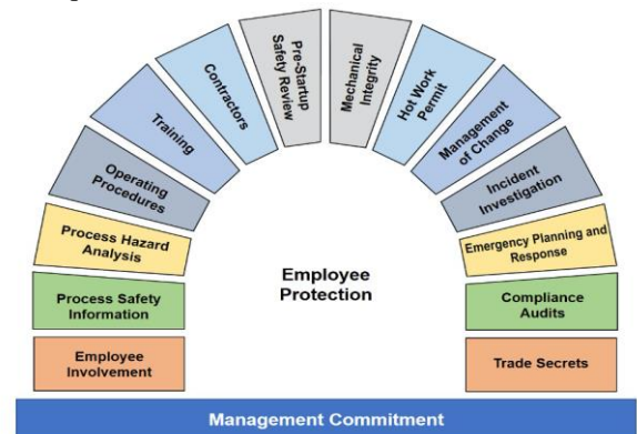
Fig – 2: PSM 14 Elements as per OSHA's Requirements
