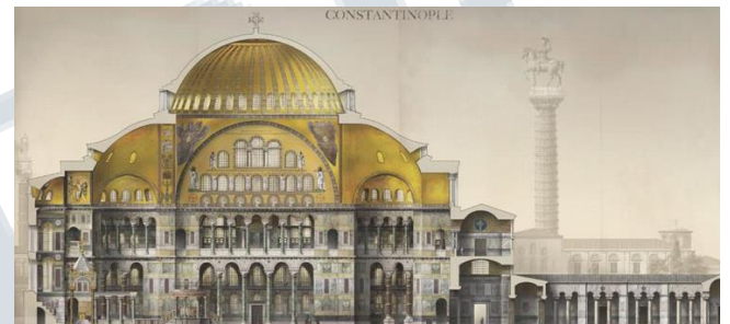
Figure 6: Section of Hagia Sophia showing the structure and the form of the main dome and semi domes
