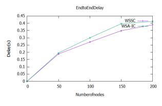
Fig.3 End-to-End Delay vs. Number of nodes Fig. 3 Presents the end-to-end delay to reach to the base station based on the number of nodes, the above simulation results determines the delay of WSSC is increased with respective of number of nodes and the performance is slightly better compare to WSA-IC for different number of nodes
