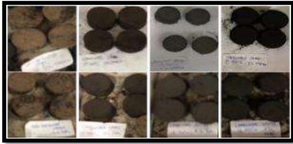
Figure 5: Different set of bio bricks developed from Water hyacinths
