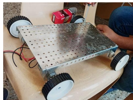
Fig 4: Fitting of Wheels and DC Motors
