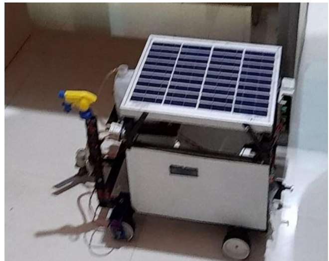
Fig 5 Solar Panel Unit of AGROBOT
