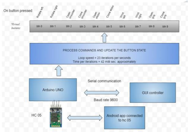
**Fig. 8. Robot control system when using the GUI interface or android blue controller.**
