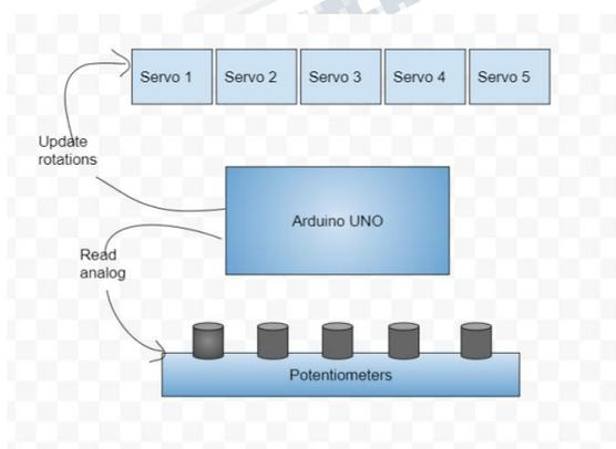
**Fig. 9. Robot control system when using the potentiometers.**
