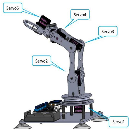
**Fig. 1. Robotic arm model & actuators**
