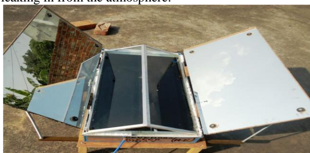
Fig. 5 Double slope solar still - working model construction
