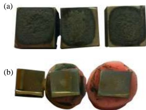
Fig.3- The image above (a) the developed microwave clad and (b) Polished Samples
