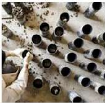
Fig.3. Sample preparation for compaction test
