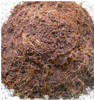
Fig. 2. Mixture of lateritic soil, coir fiber and fly ash
